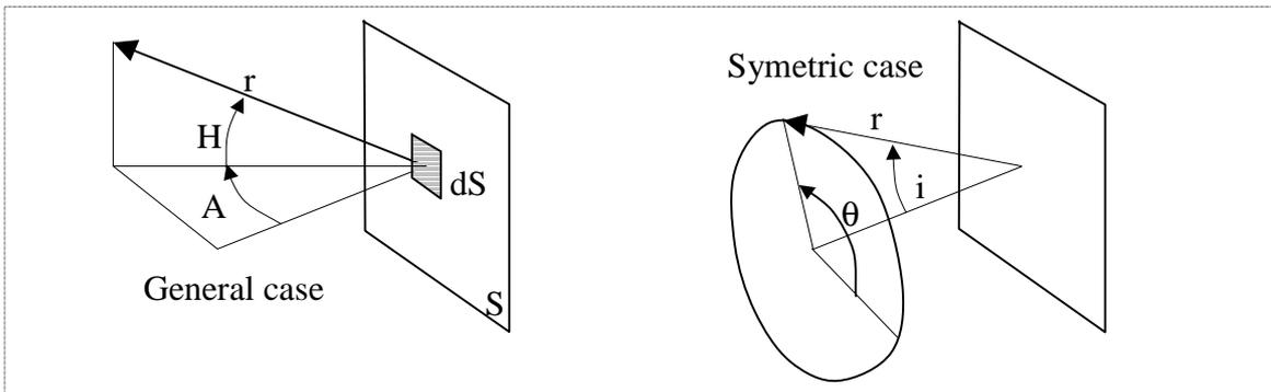
Fig. 5 : schematic description of the treatment of diffuse radiations
