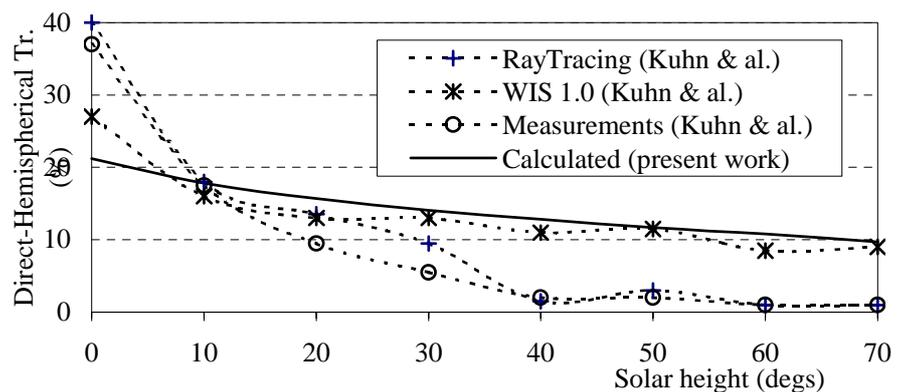
Fig. R3e : direct-hemispherical transmittance (BDT+BdT) for case 3 (internal 'daylighting' venetian blind), solar azimuth at 0°, slats at 0° (see [KUHN], fig. 12).
