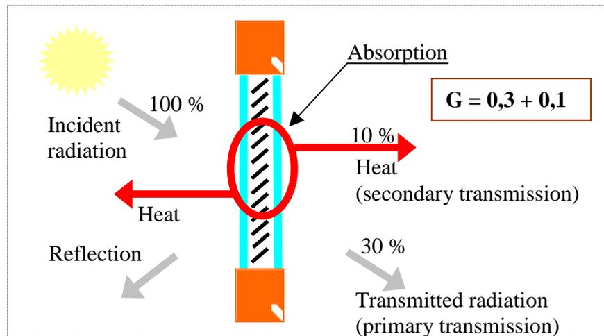
Fig. 1 : explanation of the total solar energy transmittance G-value
