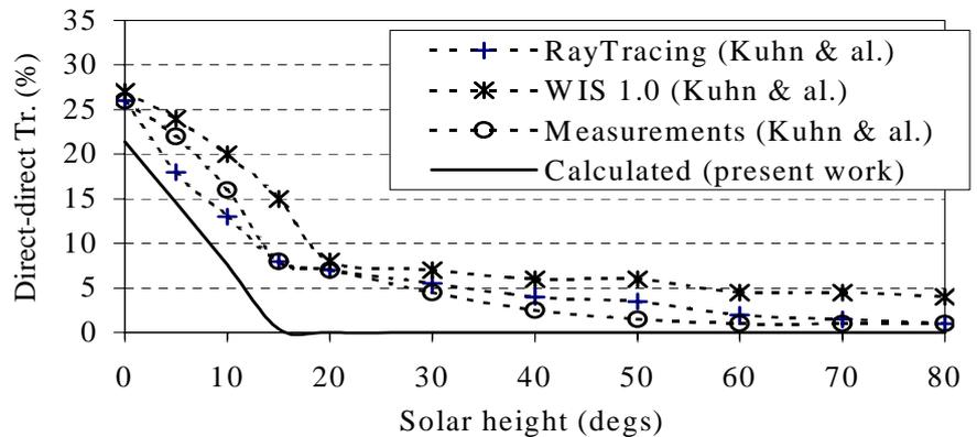
Fig R3b : direct-hemispherical transmittance (BDT+BdT), for case 1 (external venetian blind with metallic, light grey slats), solar azimuth at  $0^\circ$ , slats at  $0^\circ$  (see [KUHN], fig. 9).
