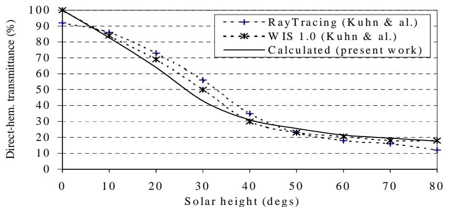
Fig. R3d : direct-hemispherical transmittance (BDT+BdT) for case 3 (internal 'daylighting' venetian blind), solar azimuth at  $0^\circ$ , slats at  $45^\circ$  (see [KUHN], fig. 11).
