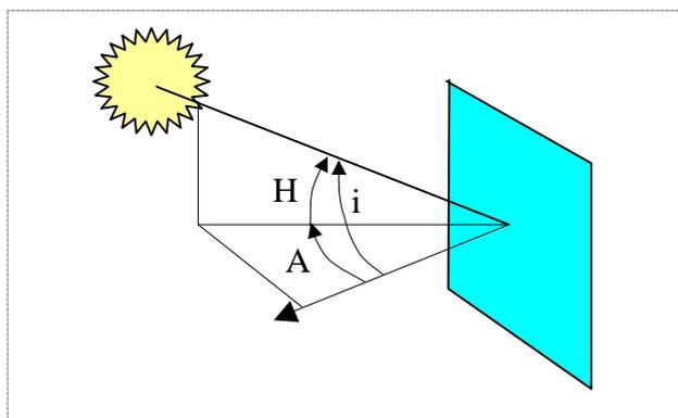
Fig. 2 : schematic description of solar angles
