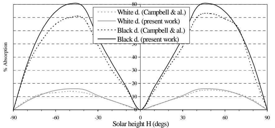
Fig. R2d : direct absorptance (BDA), for slats at 45°
