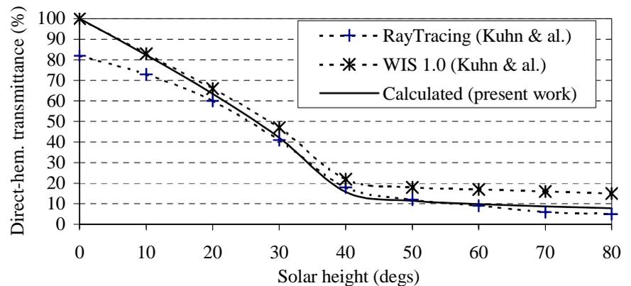
Fig. R3c : direct-hemispherical transmittance (BDT+BdT), for case 2 (internal venetian blind with perforated white slats), solar azimuth at  $0^\circ$ , slats at  $0^\circ$  (see [KUHN], fig. 10).
